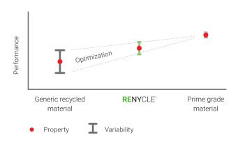
3033BK (PA6-GF30 whose PA6 polymer is recycled). What can be seen is that as the recycled content increases, although the design of the materials aims at maintaining the properties, there is a reduction in performance compared to the first choice which is not negligible. This aspect, of fundamental importance, must be taken into consideration in the component design phase when implementing the criteria for choosing the materials.
