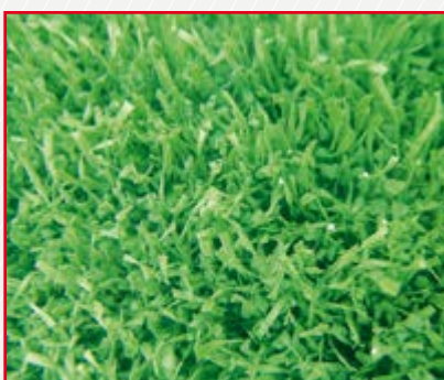
RADIGREEN® HDF PE AFTER 40,200 LISPORT CYCLES
