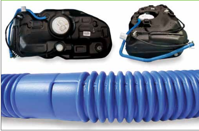
Figure 5 | Tank breather hose made of Radilon® D 40EP25ZW 7037 BL.
