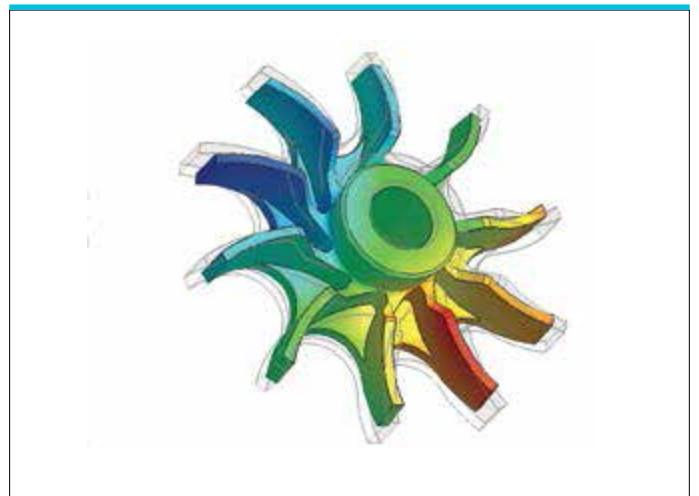
Figure 3 | Warpage prediction for a pump impeller (magnified scale).
