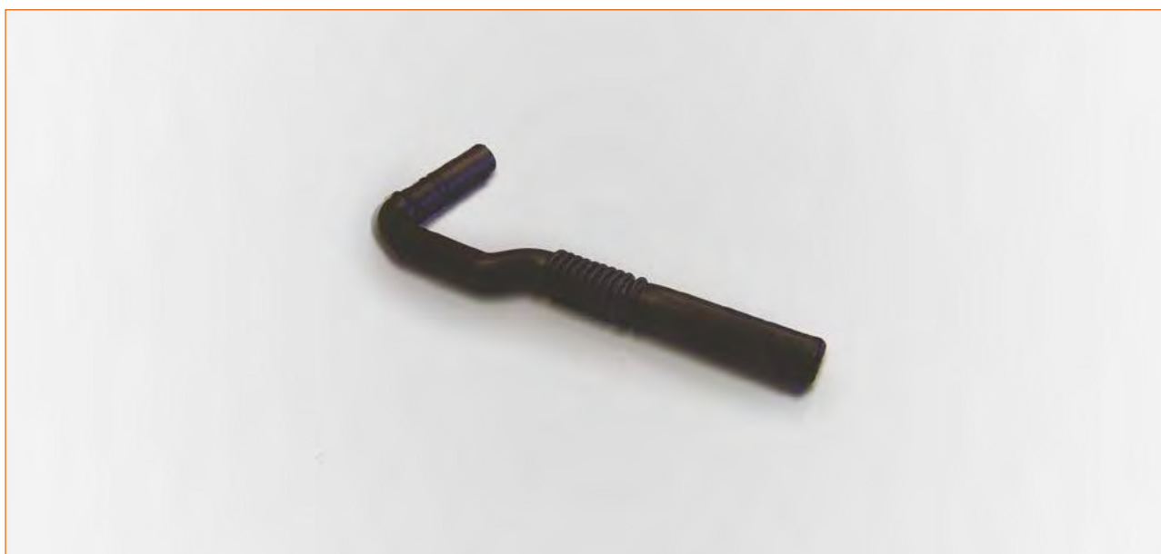
FIG.9 - TURBO AIR DUCT MADE FROM RADILON® A BMV200 HHR USING SUCTION BLOW MOULDING
