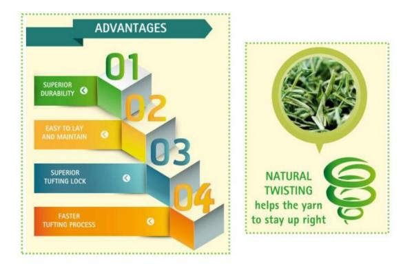
TPR production technology produces clean and precise fibrillation, which is essential to prevent the fibre from weakening. RADIGREEN® HD PE yarn can withstand prolonged stress because of its self-twisting property, a helix effect that strengthens the yarn by increasing resilience and split resistance.
