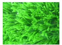
from weakening. RADIGREEN® HD PE yarn can withstand prolonged stress by developing a self-twisting property, a helix effect that strengthens the yarn by increasing resilience and split resistance.
